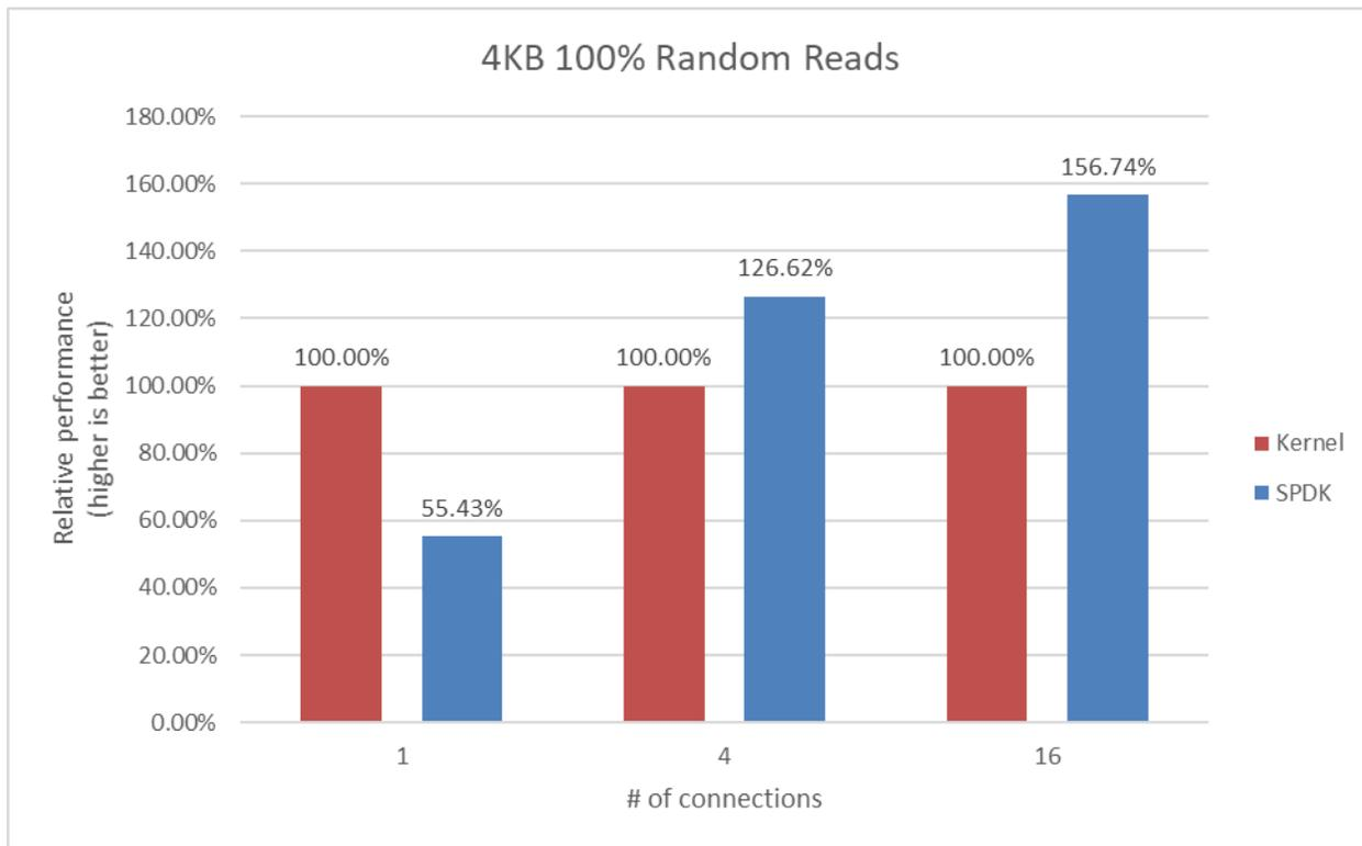
Figure 14: Relative Efficiency Comparison of Linux Kernel vs. SPDK NVMe-oF Target IOPS/Core for 4KB 100% Random Reads QD=128 using the Kernel Initiator
