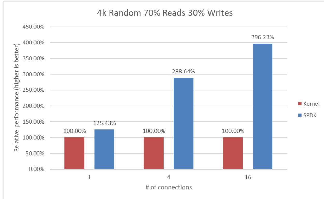
Figure 13: Relative Efficiency Comparison of Linux Kernel vs. SPDK NVMe-oF RDMA Target IOPS/Core for 4KB Random 70% Reads 30% Writes QD=128 Workload, using Kernel Initiators
