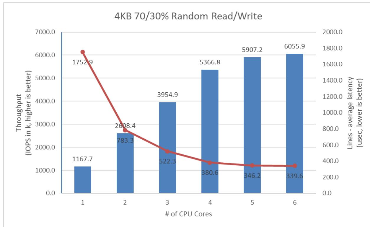
Figure 4: SPDK NVMe-oF RDMA Target I/O core scaling: IOPS vs. Latency while running 4KB Random 70/30 Read/Write workload at QD=128
