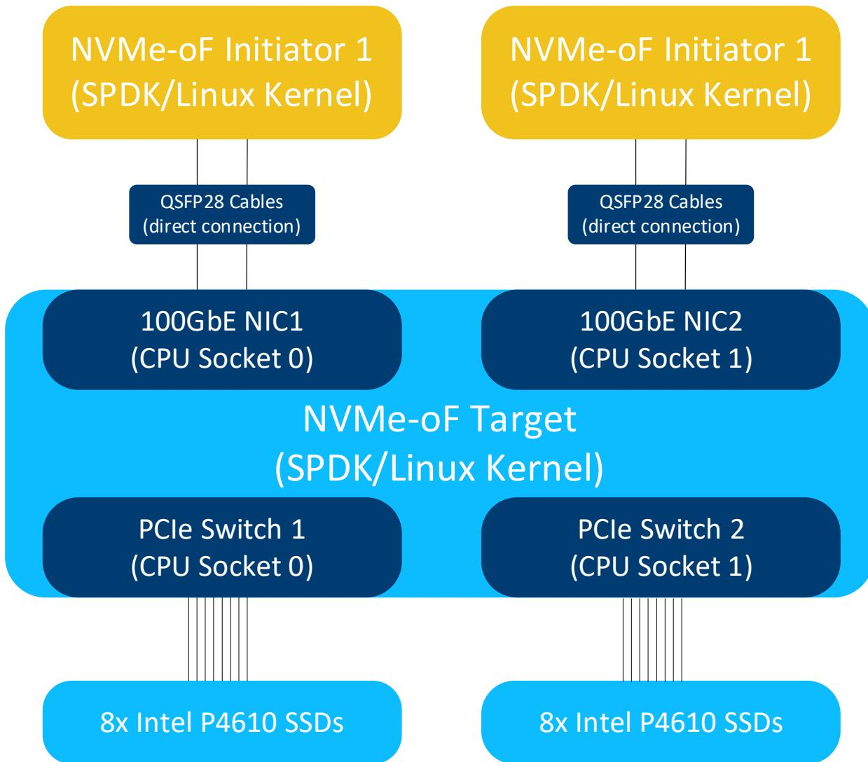
Figure 1: High-Level NVMe-oF RDMA performance testing setup
