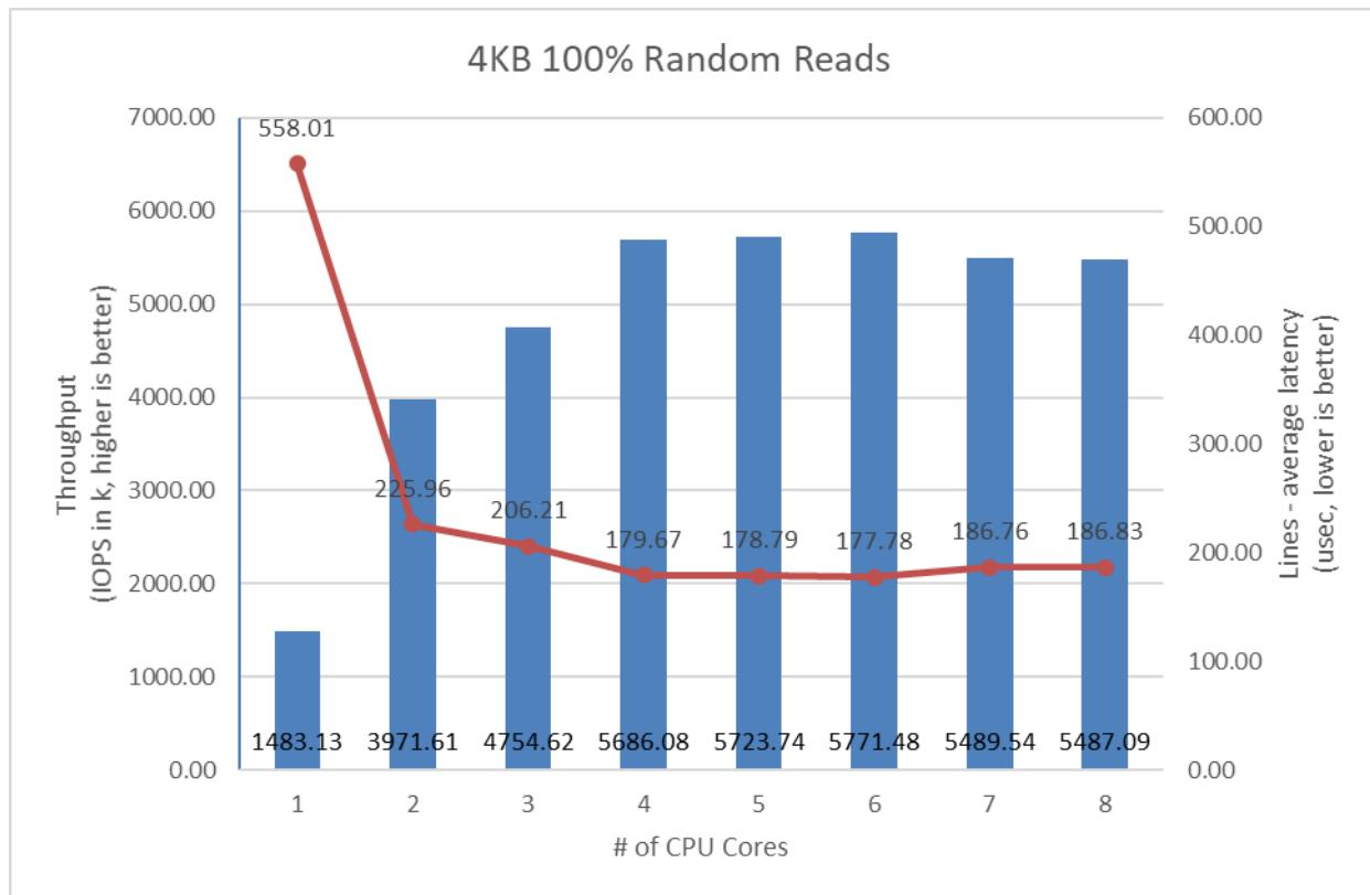
Figure 5: SPDK NVMe-oF RDMA Initiator I/O core scaling: IOPS vs. Latency while running 4KB 100% Random Read workload at QD=64
