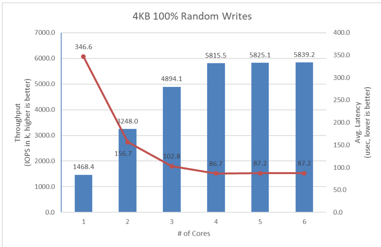
Figure 3: SPDK NVMe-oF RDMA Target I/O core scaling: IOPS vs. Latency while running 4KB 100% Random Write workload at QD=32
