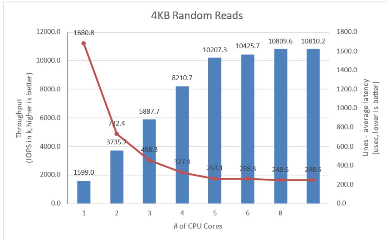
Figure 2: SPDK NVMe-oF RDMA Target I/O core scaling: IOPS vs. Latency while running 4KiB 100% Random Read workload at QD = 192
