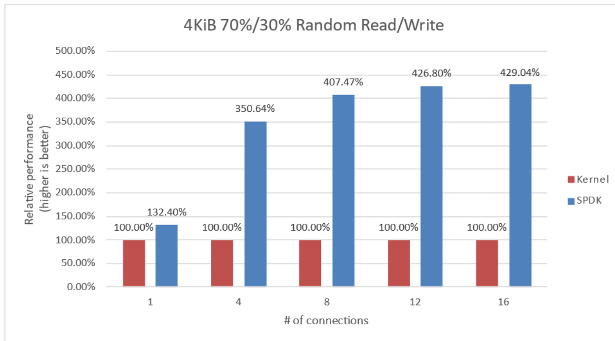
Figure 13: Relative Efficiency Comparison of Linux Kernel vs. SPDK NVMe-oF RDMA Target IOPS/Core for 4KiB Random 70% Reads 30% Writes QD=192 Workload, using Kernel Initiators
