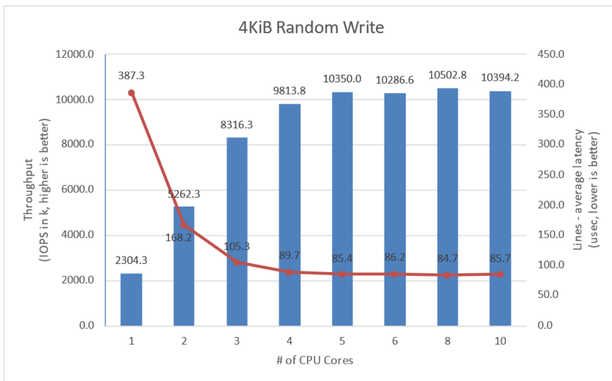
Figure 3: SPDK NVMe-oF RDMA Target I/O core scaling: IOPS vs. Latency while running 4KiB 100% Random Write Workload at QD=64
