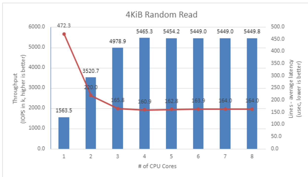
Figure 5: SPDK NVMe-oF RDMA Initiator I/O core scaling: IOPS vs. Latency while running 4KiB 100% Random Read QD=64 workload
