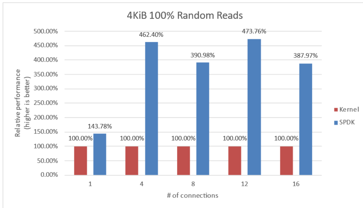
Figure 11: Relative Efficiency Comparison of Linux Kernel vs. SPDK NVMe-oF RDMA Target IOPS/Core for 4KiB 100% Random Reads QD=192, using the Kernel Initiator
