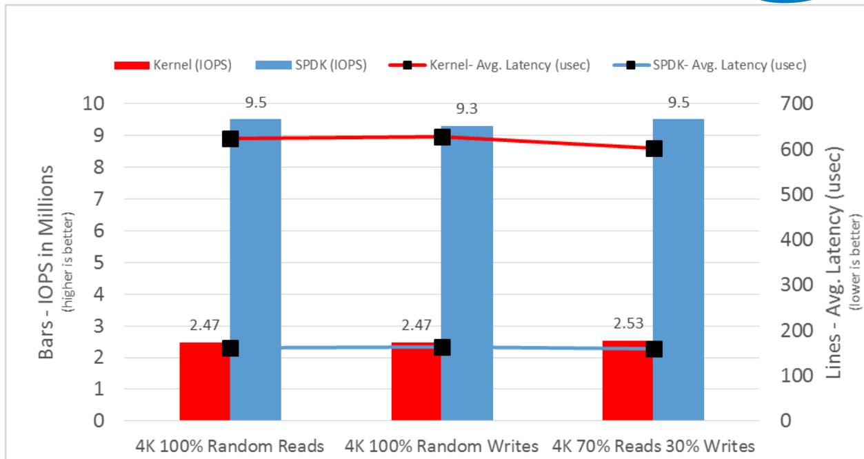
Figure 10: Kernel vhost-scsi vs. SPDK vhost-scsi target: IOPS vs. Avg. Latency for various I/O workloads using 10 vhost-scsi cores
